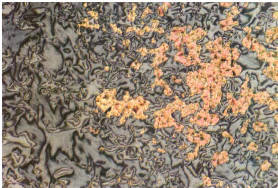
Plate 5. The focal conic fan and schlieren optical textures of the smectic C phase exhibited by 10.O6O.10 ( T = 160^{\circ}\text{C} ).
