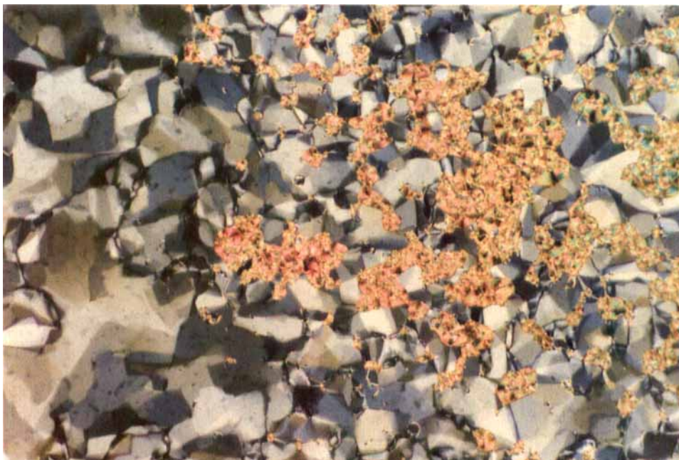
Plate 6. The optical texture of the smectic F phase obtained on cooling the smectic C phase of 10.O6O.10 in plate 5 ( T = 115^{\circ}\text{C} ).
